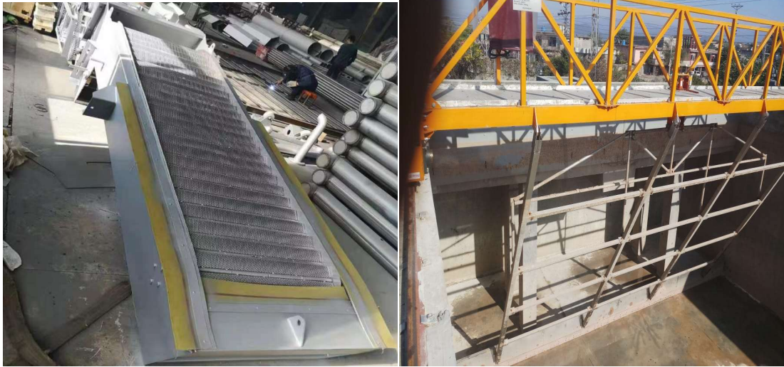
Vertical mechanical screen and to and fro scrapper fabricated in our workshop
